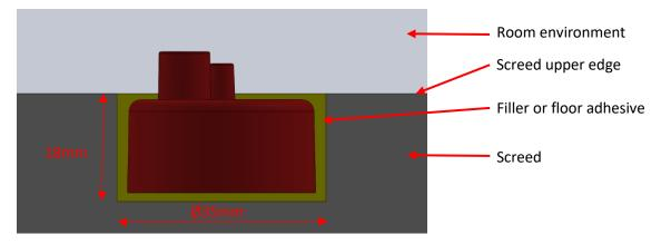
With both variants it is very important that no screed/filler or adhesive enters the openings on the top of the easylogger, otherwise the measurement result will be falsified.
